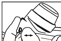
Figure 3 – Vacuum release lever
